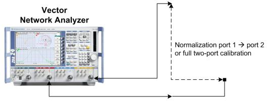
Fig. 1-2: VNA test setup for cable calibration
