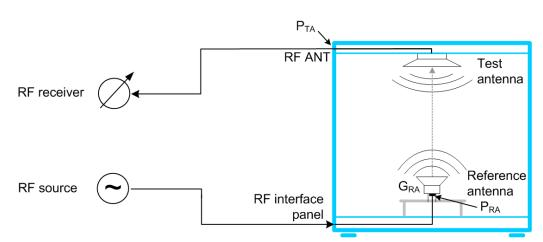
Fig. 1-1: Schematic test setup for reference path loss measurement
